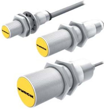
Cylindrically shaped capacitive sensors feature high switching distances and are available in a vast range of types. M12, M18 and M30 chrome-plated threaded barrels are available with connection cable or plug connection. Besides the usual reliability, capacitive sensors feature standard properties such as automatic wetting compensation, excellent EMC and ESD properties and more flexibility with respect to mounting.
