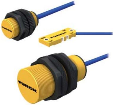
NAMUR sensors are approved for the zones 0 and 1. They are polarized 2-wire devices, changing their internal resistance in dependence on the attenuation (continuous linear/current characteristics). They can be connected to external switching amplifiers which convert current variations into binary output signals. The advantage: With an approved switching amplifier, they can be applied in Ex-areas as well as monitor wire-break and short-circuit continuously.
