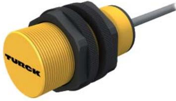
The BCC sensors blank out all interferences during the monitoring process and feature excellent EMC and ESD properties. A laterally mounted shield and an integrated processing unit inhibit predamping when mounted in metal flanges. The full switching distance is thus available.
