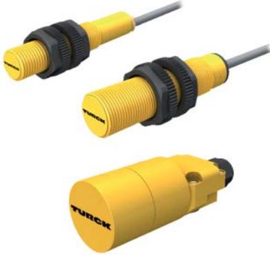
Cylindrically shaped capacitive sensors feature high switching distances and are available in a vast range of types. The standard types come in plastic housings and sizes from Ø 12 mm to Ø 40 mm, with connection cable, plug connection or terminal chamber.
