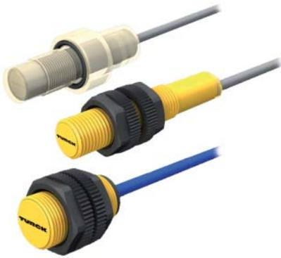
A growing number of applications require sensors resisting temperatures beyond the standard range of -25 ... +70 °C. For this purpose TURCK has developed capacitive sensors which meet exactly these requirements. The sensors feature temperature resistant components as well as cleverly designed passive cooling concepts, approved in demanding laboratory tests. These sensors resist temperatures from -25 °C to +100 °C.
